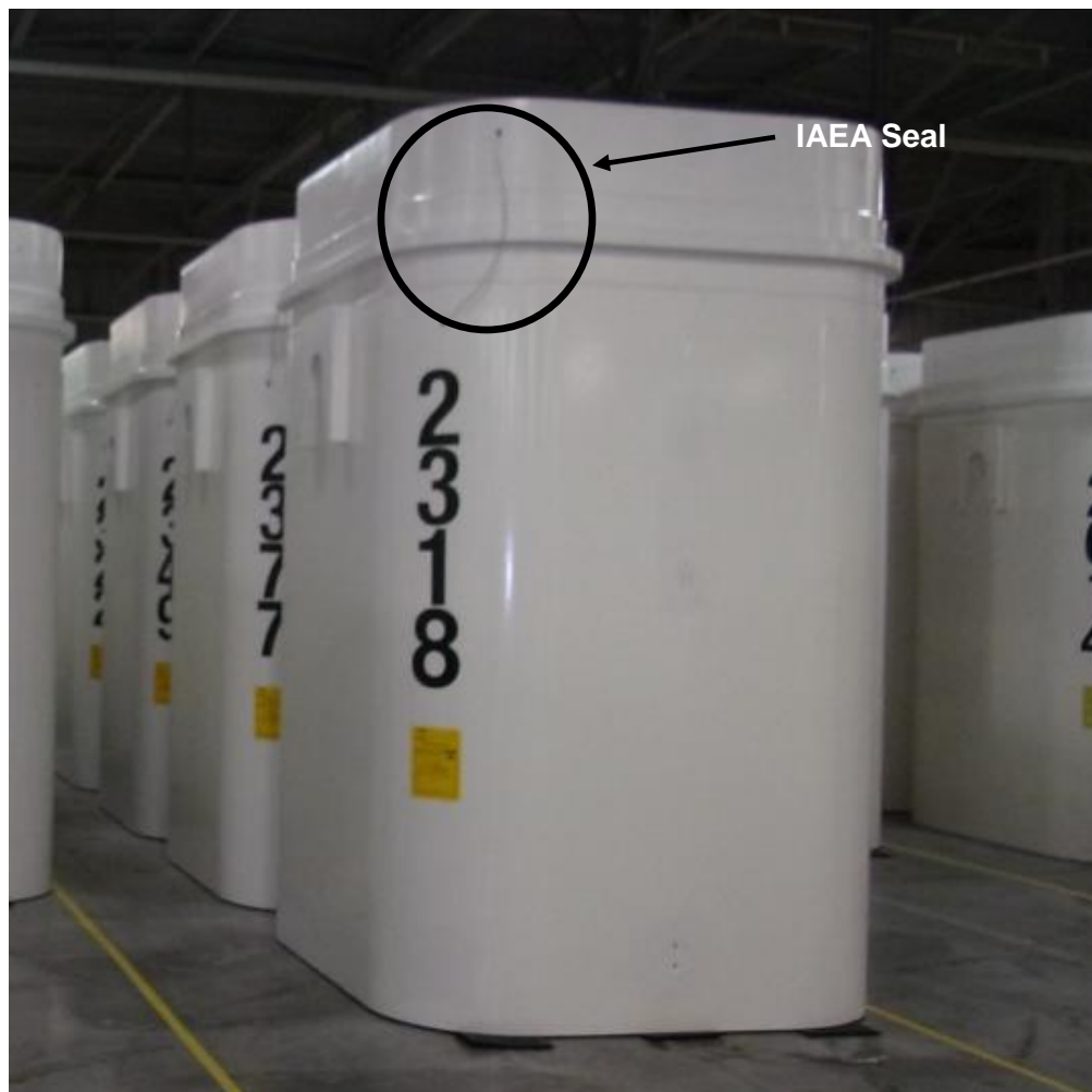
Figure 19: DSCs in Storage with IAEA Wire Seals
